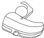
Now place the battery in the battery compartment with the golden side facing upwards and close the battery compartment.
