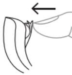
To turn the hearing aid on, close the battery door. The hearing aid will play a sound signal to indicate that it is on, unless your hearing care professional has deactivated this function.
